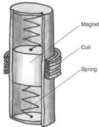
Fig. 1. An electromagnetic generator envisaged to generate UV radiation
