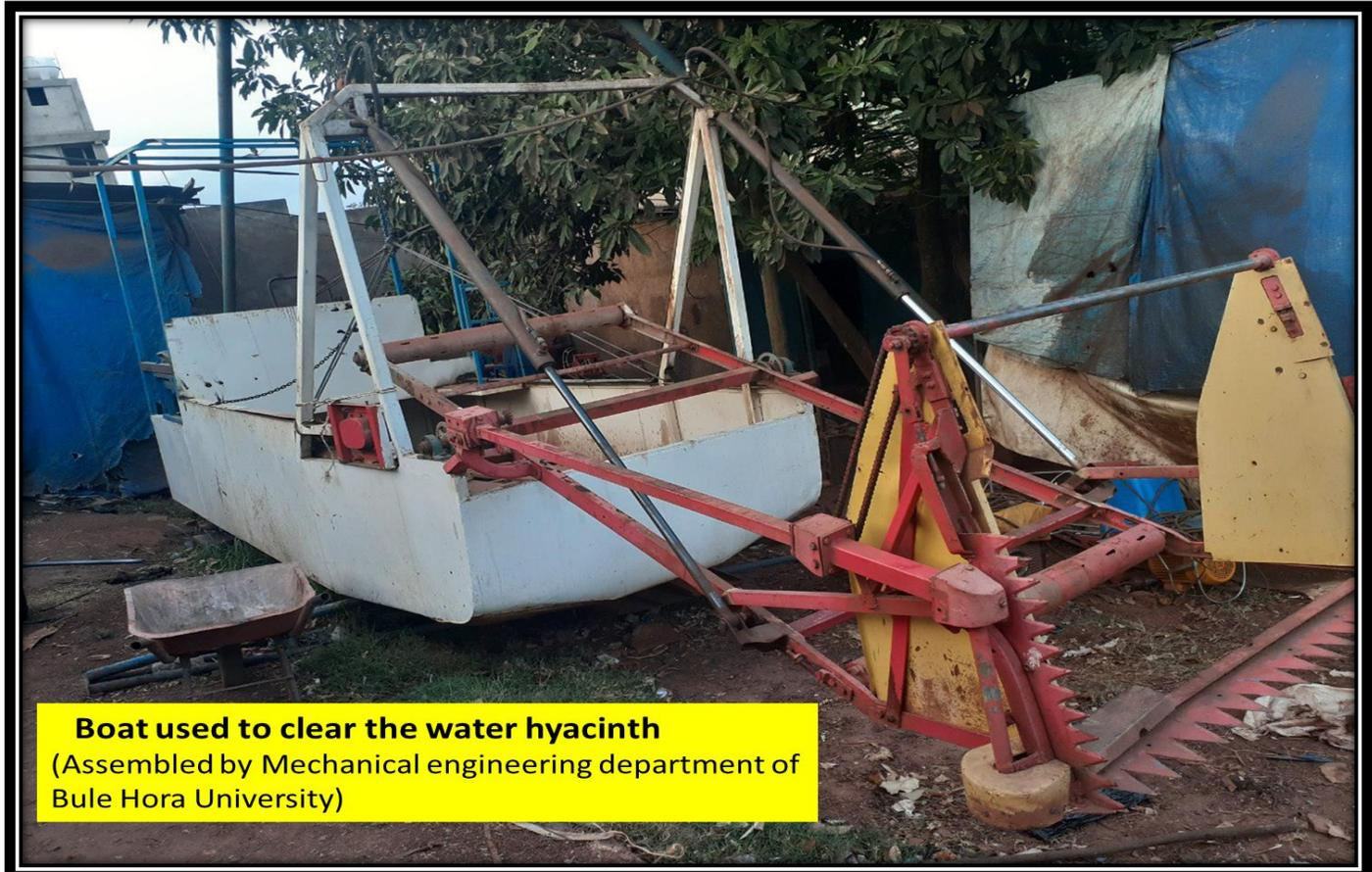
Fig. 4. A boat prepared to remove water hyacinth from Abaya Lake
